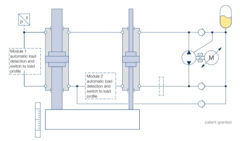
The control by servo pumps and the load-controlled automatic transmission switch through the modules 1 and 2 enable a minimum necessary volume flow and thus the use of small internal gear pumps and servomotors as well as smaller servo converters. In addition to the resulting dynamics advantages, this means less space is required and the budget is relieved.
